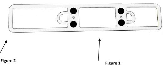
Install side frame with long frame extension towards the front of radio.
